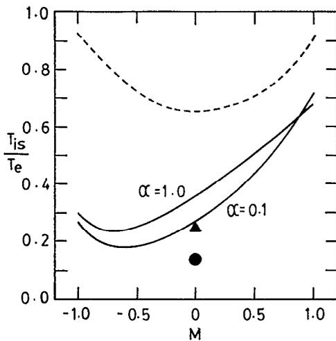
FIG. 5. Sheath ion temperatures ( $T_{is}$ ) with different drifts ( $M$ ) and viscosity contributions ( $\alpha$ ). Solid lines are from the kinetic model for  $\alpha = 1.0$  and 0.1, and the broken line is from the fluid model with energy equation for  $\alpha = 1.0$ ,<sup>15</sup> ▲: from Emmert *et al.*,<sup>6</sup> ●: from Bissel and Johnson,<sup>7</sup> which are equivalent to  $\sigma_i = 0$  with different ionization source types.
