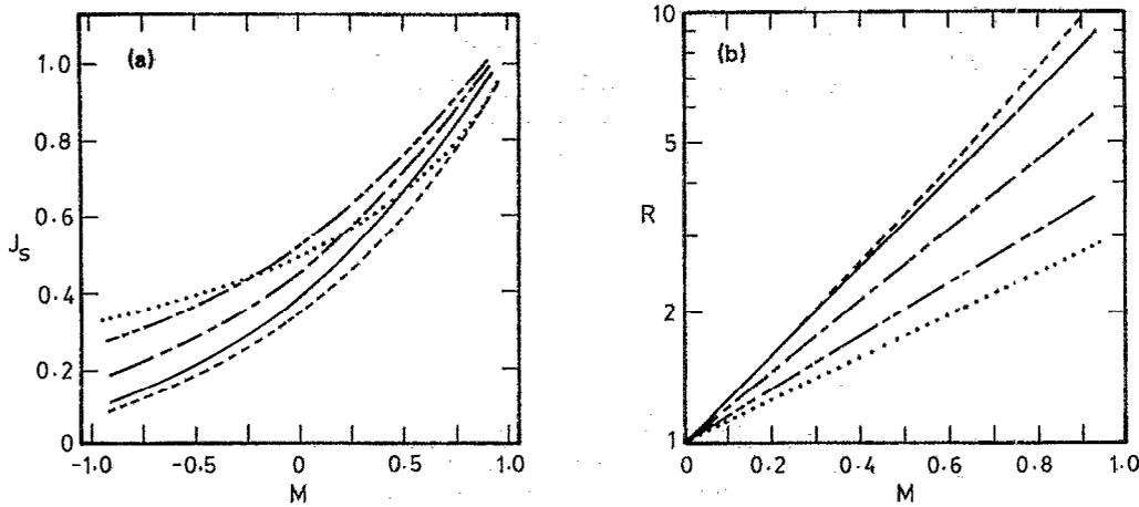
FIG. 2. Sheath current densities (a) and ratios (b) for different viscosity contributions. [ $\alpha = (\dots)0.0$ ,  $(- \cdot -)0.5$ ,  $(- -)1.0$ , with  $-1 < M < 1$  and  $T_{i\infty} = T_e$ . Comparison is made with fluid models Hutchinson<sup>11</sup>  $(- \cdot -)$  and Stangeby<sup>10</sup>  $(\dots)$ ].
